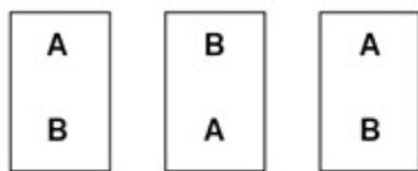
**NOTE:** To allow for free movement of spray arms when loading more than one Bottom Rotary Spray Header side-by-side in the washer/dryer, loading direction of every-other header must be reversed as shown. A and B designate the rotary spray arms.
